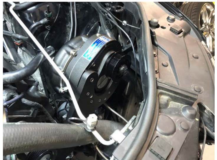
Procharger Head Unit Installed
