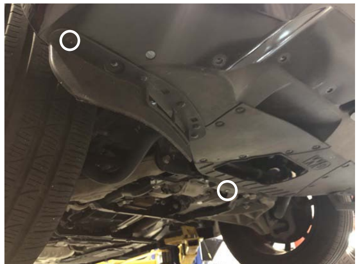
Push Pin and Rivet
