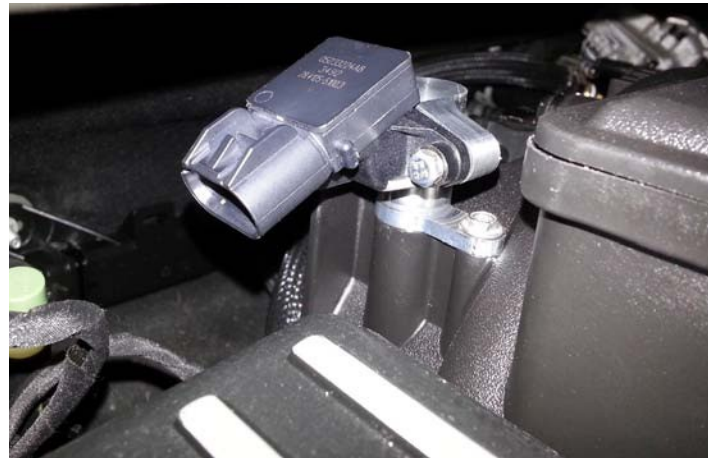
New MAP Sensor Installed
