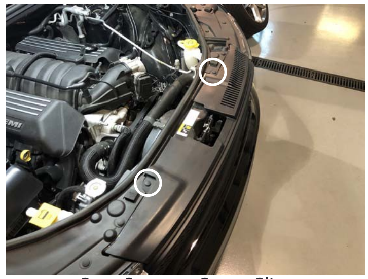
Core Support Cover Clips
