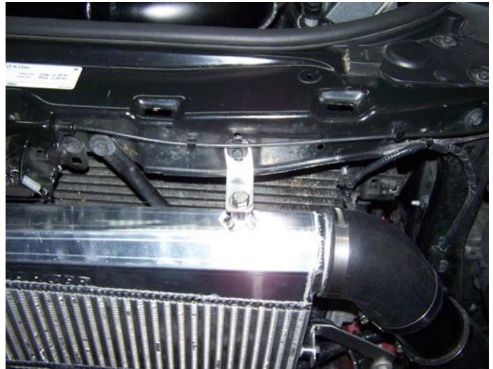
Driver's Side Intercooler Mounted
