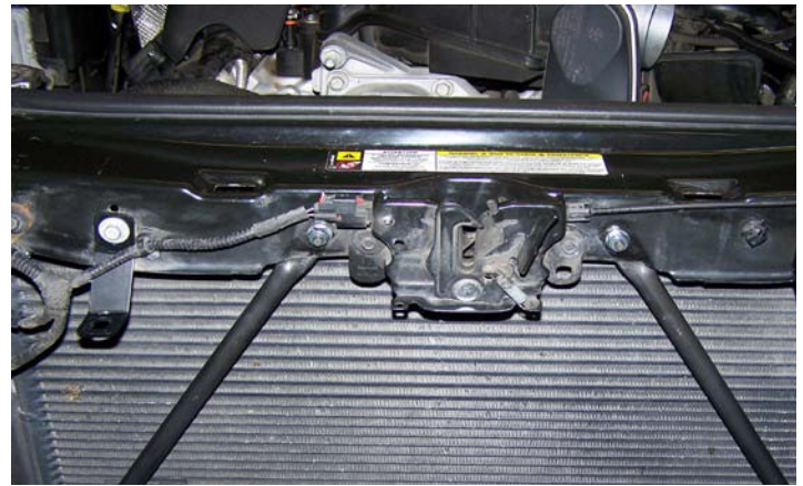
Radiator Support Brackets Relocated
