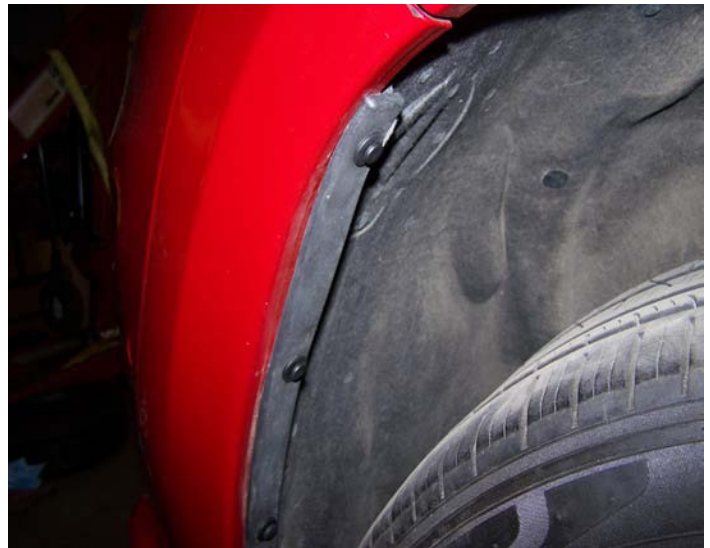
Wheel Liner Push Pins (Jeep)
