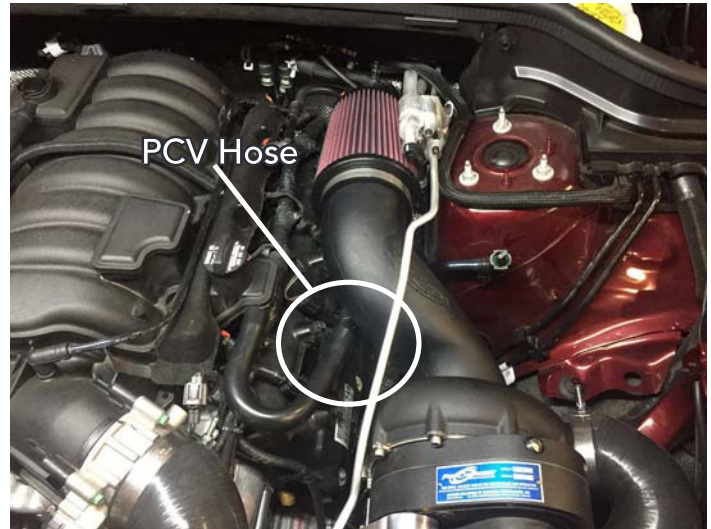
Air Inlet Installed
