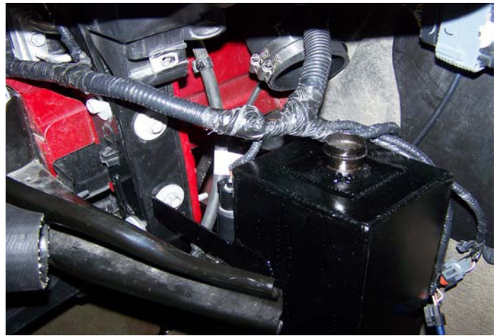
Washer Tank Installed
