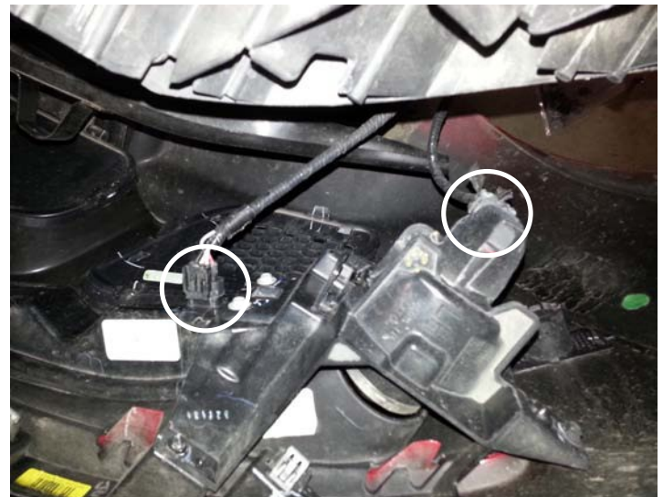
Fog Light & Turn Signal Connectors (Drivers)
