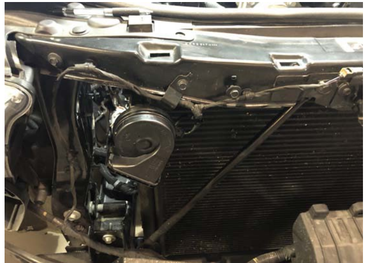
Passenger Side Horn Mounted
