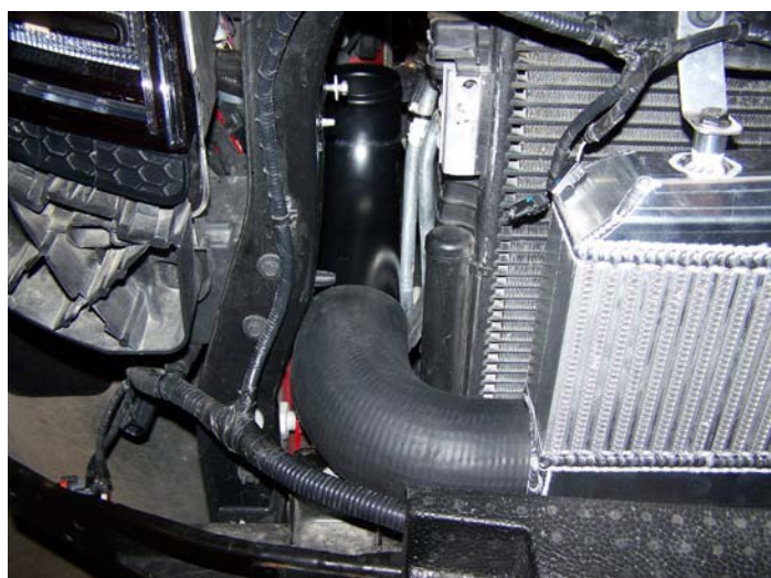
Tubing Out Of The Intercooler Installed
