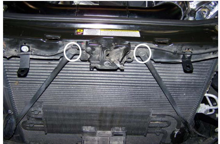
Radiator Support Brackets
