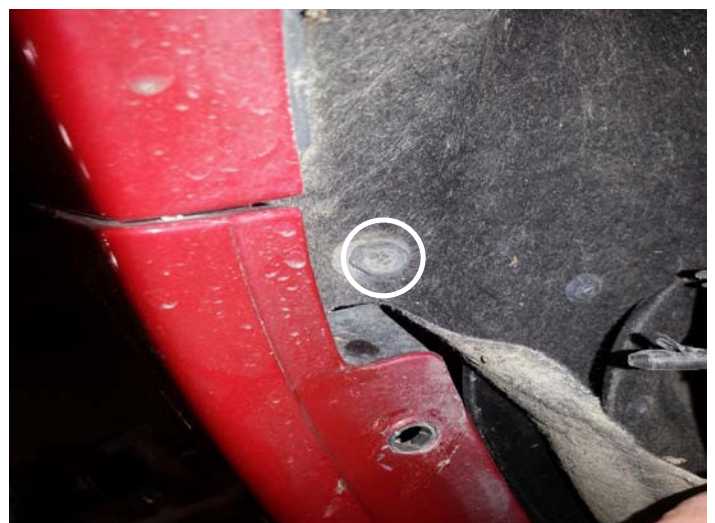
Wheel Liner Bolt
