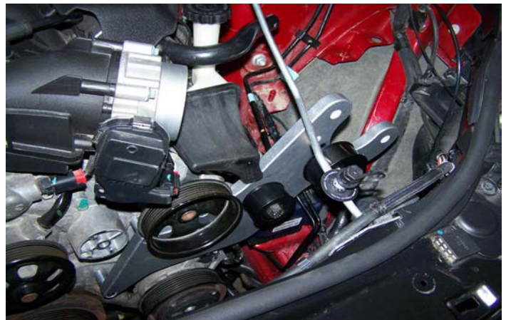
Main Bracket Installed
