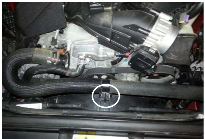
Radiator Hose Hold Down Clamp
