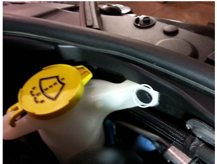
Plastic Clip At Fill Cap
