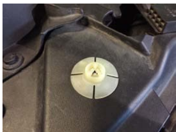
Transmission cooler Back Clip
