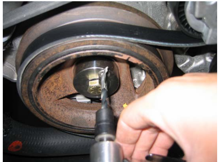
Drilling the Crank
