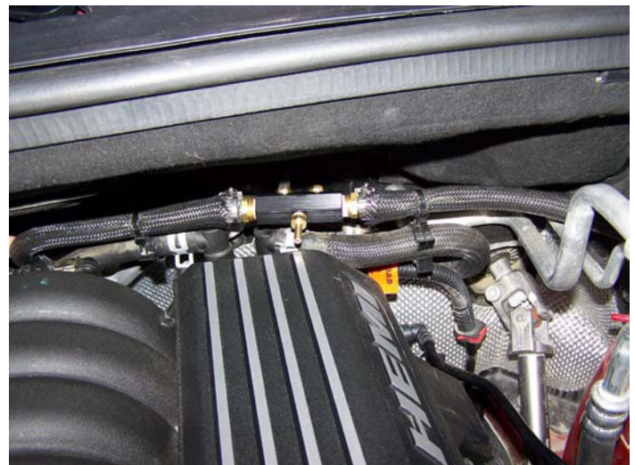
Vacuum Manifold Installed
