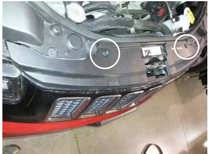
Core Support Cover Clips
