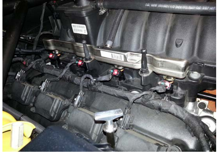
Fuel Rails Installed
