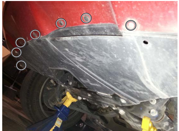
Fascia Screws & Clips (7 Of 9 Shown)
