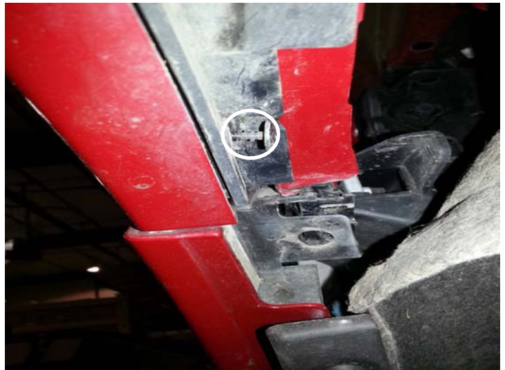
Fender To Fascia Screw (2012-16 Models)
