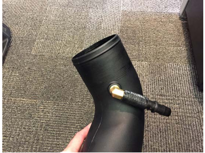
Fitting, Rubber Hose and Plastic Reducer Installed Onto Inlet
