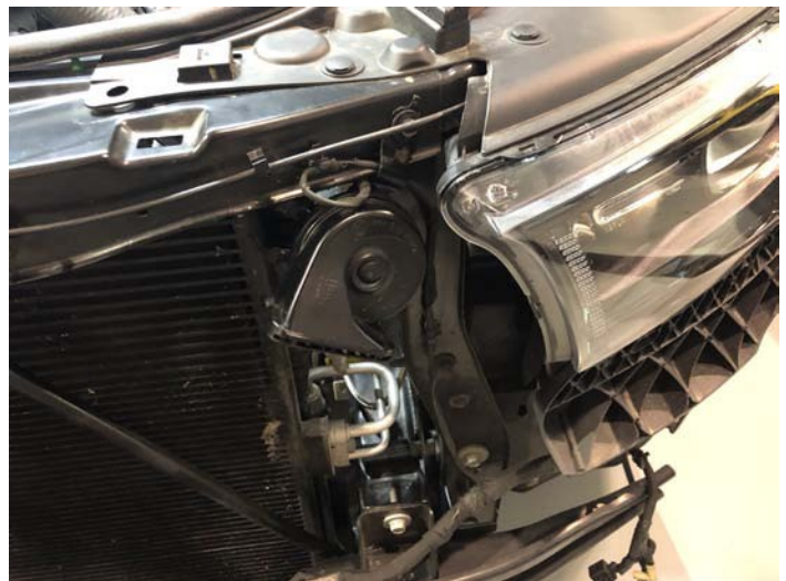
Driver's Side Horn Mounted
