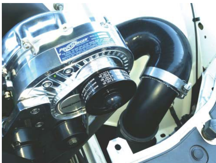
Blower Discharge Connection
