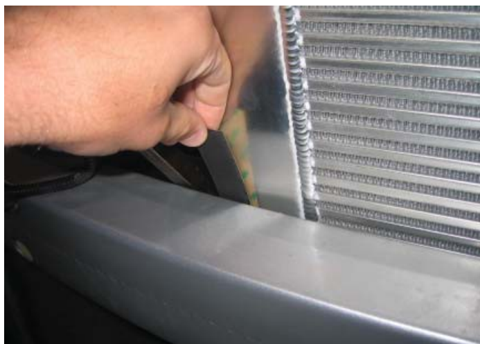
Place Tape Between Intercooler and Front Bumper for Insulation
