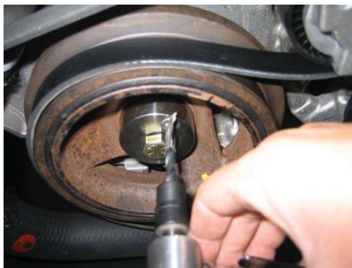
Drilling the Crank
