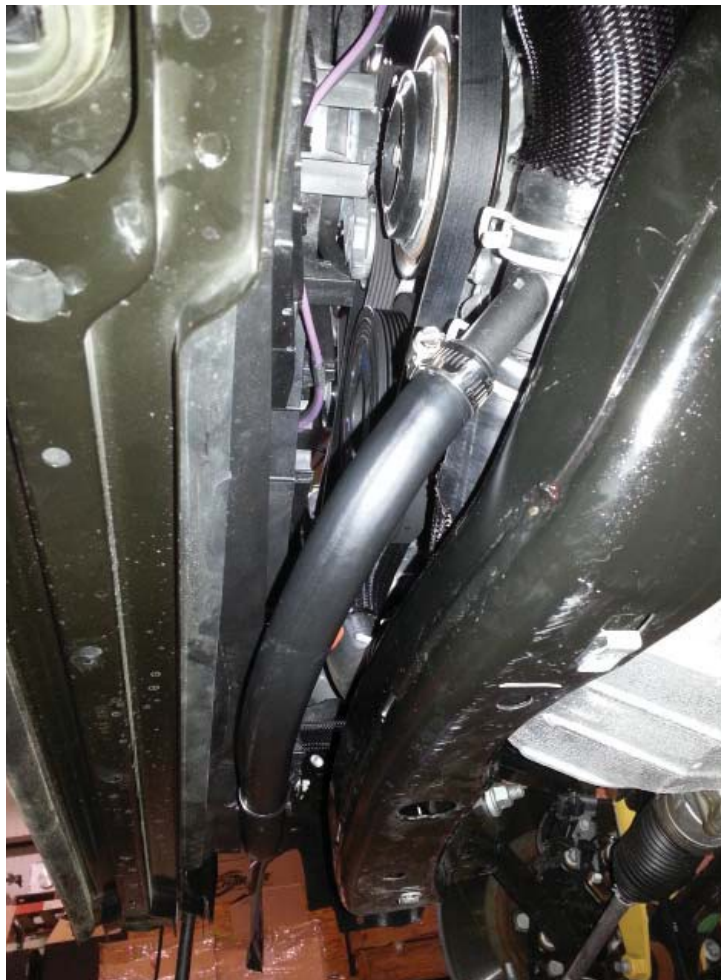
New Coolant Hose Routed (6.4L)
