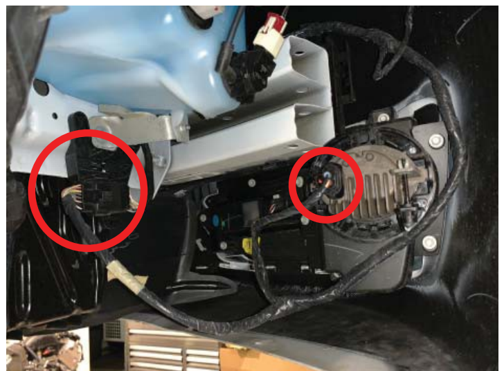
Unplug Wiring Harness
