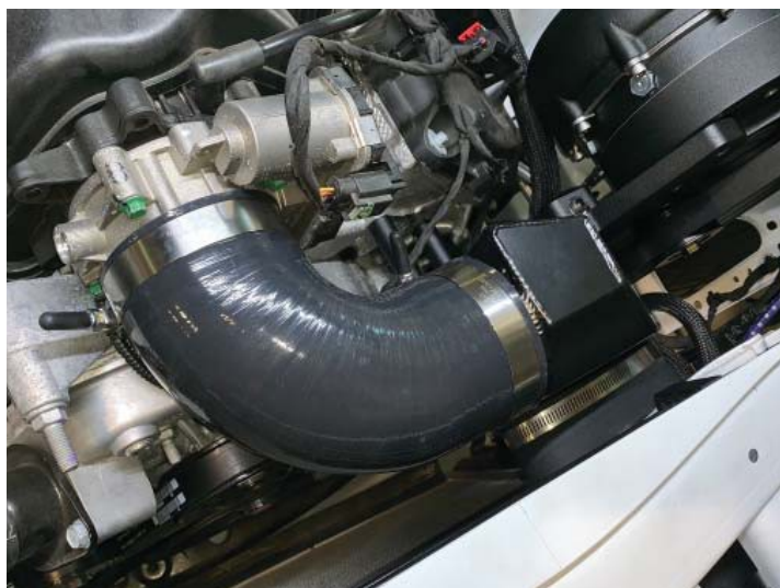
Throttle Body Tube Installed
