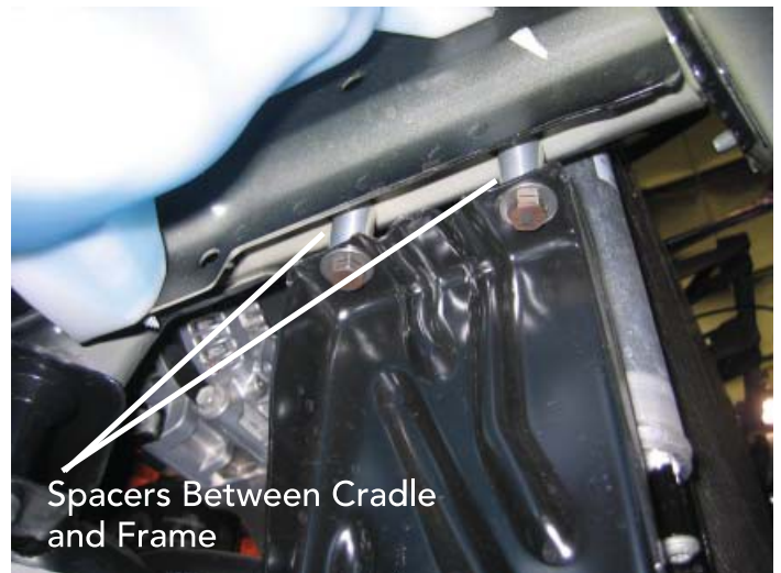
Radiator Cradle Spacing (Pass. Side)
