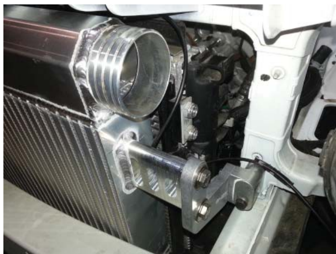
Driver's Side Intercooler Brackets
