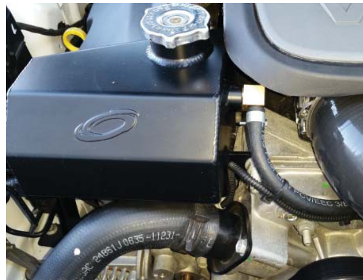
Coolant Hoses Connected
