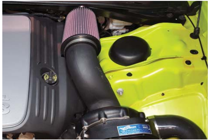
Cover Trimmed for Air Inlet
