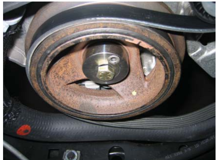
Drill Jig Installed
