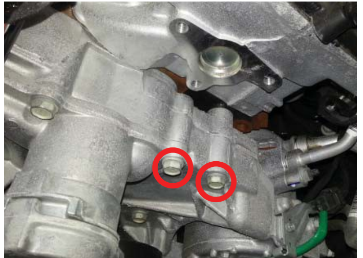
Remove Timing Cover Bolts
