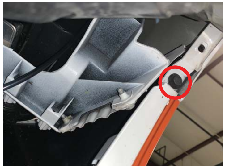
Wheel Well Bumper Bolt
