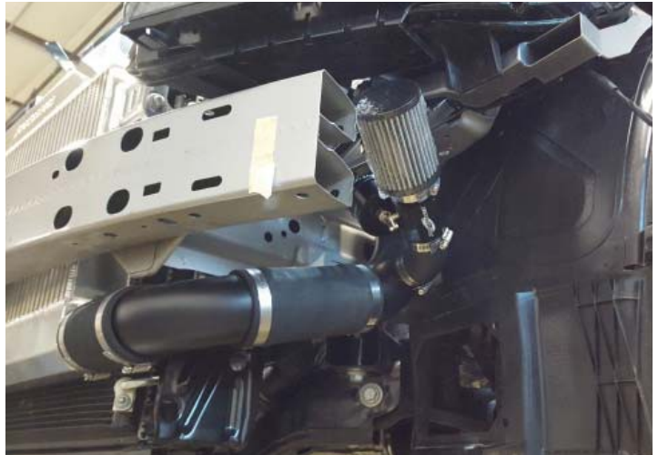
Surge Valve Installed
