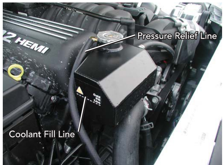
Pressure Relief Line Routing and Fill Line
