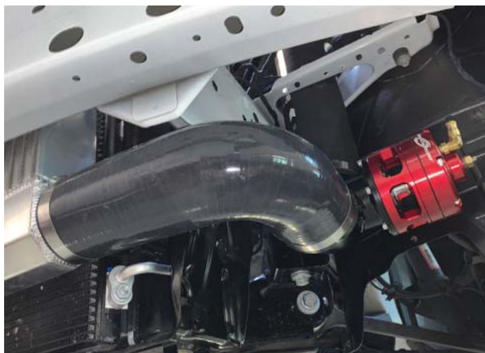
Race Intercooler Connection
