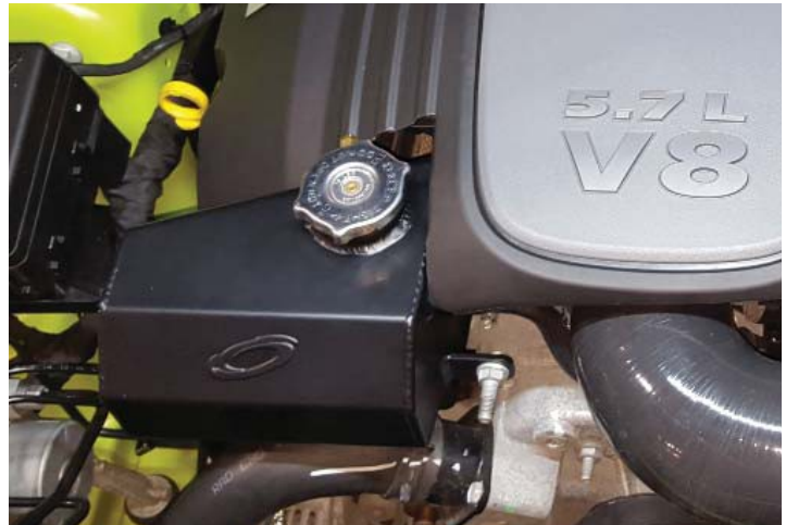
Cover Trimmed for Coolant Reservoir
