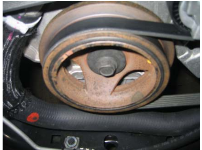
Factory Crank Pulley and Bolt
