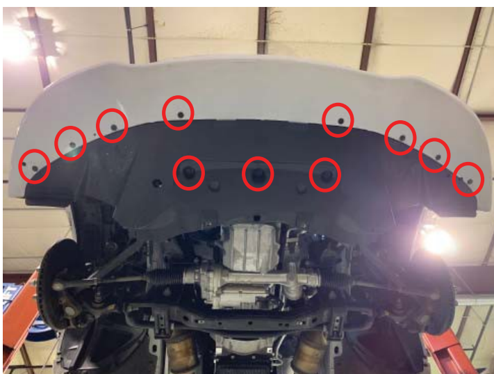
Remove Front Cladding
