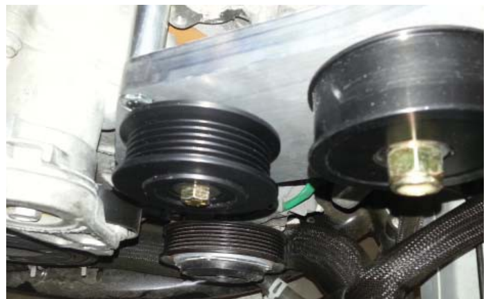
Ribbed Idler Installed
