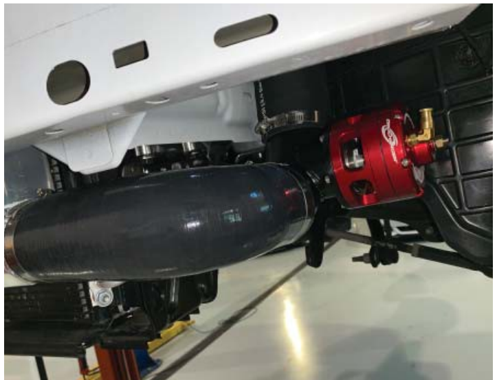
Optional Race Valve Installed
