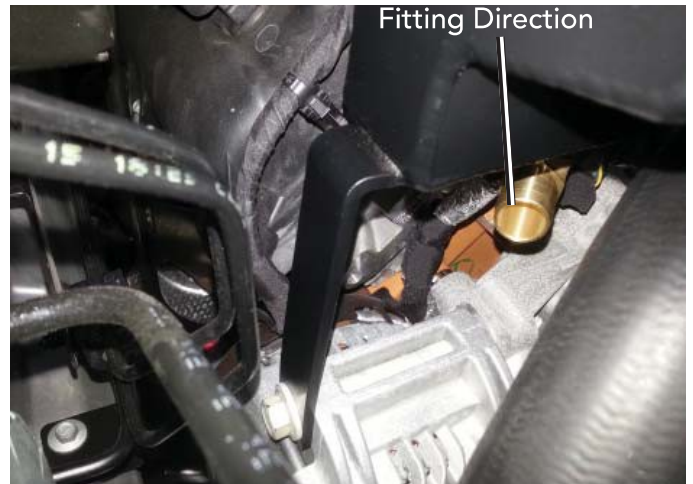
3/4" Brass Fitting Direction
