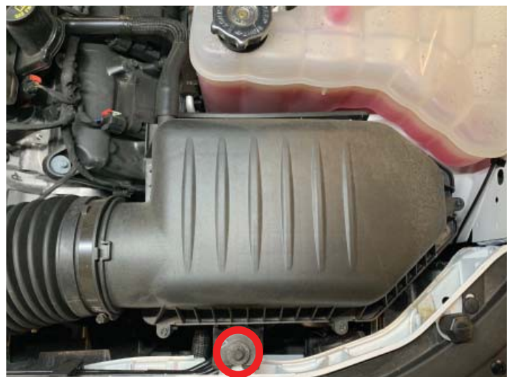
Remove Air Filter Assembly Bolt
