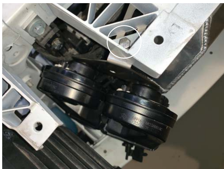
Pass. Side Intercooler & Horn Relocation
