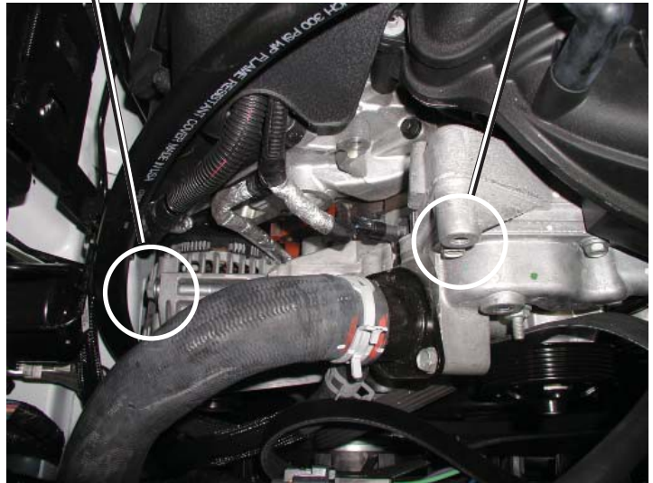
Coolant Reservoir Mounting Locations
