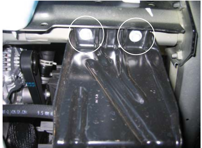
Radiator Cradle Bolts (Pass. Side)
