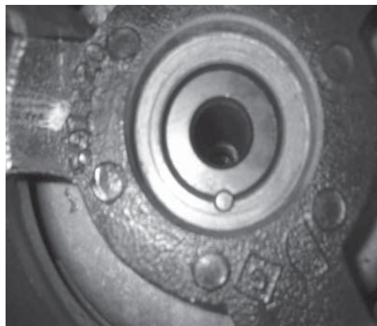
Crank Pulley Pinned to Crankshaft
