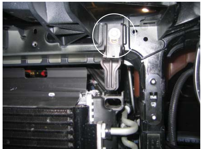
Radiator Upper Mount Bolts (Driver's Side)
