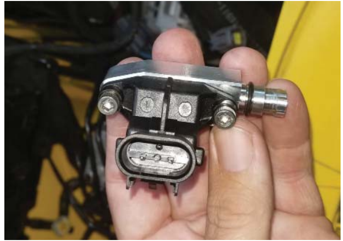
MAP Sensor Installed
