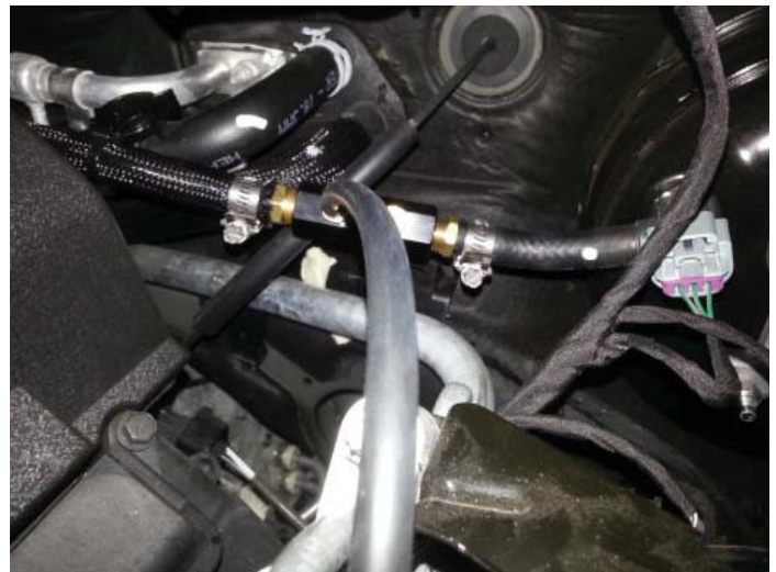
Vacuum Manifold Installed
