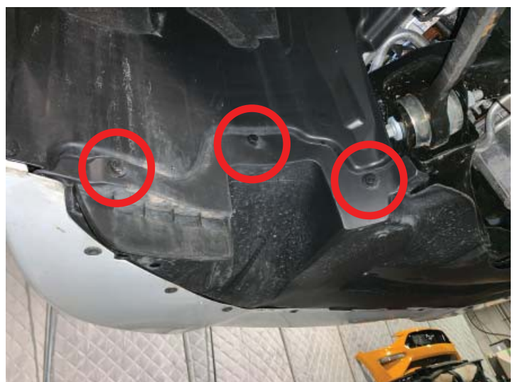
Remove Front Cladding
