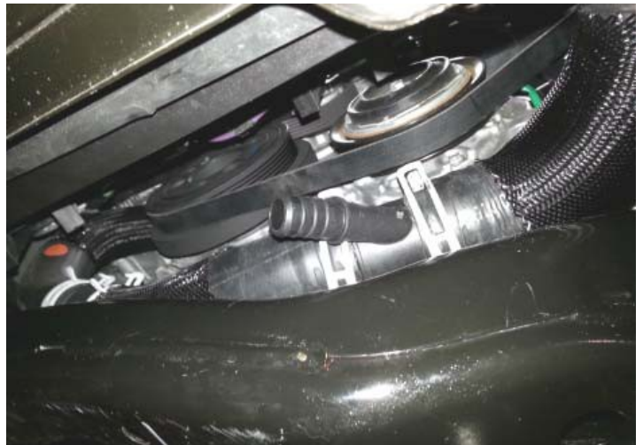
Coolant Fitting Reversed (6.4L)
