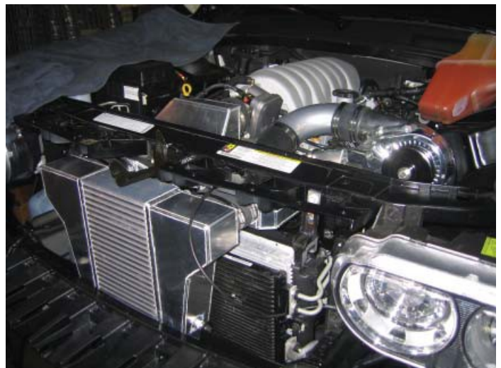
Intercooler and Tubing Installed
