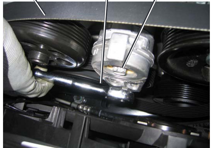
Factory Belt and Tensioner Removal
