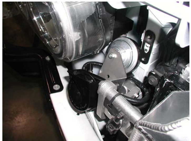
Pass. Side Intercooler & Horn Relocation
