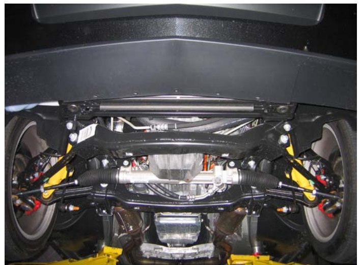
Underside Body Cladding Removed
