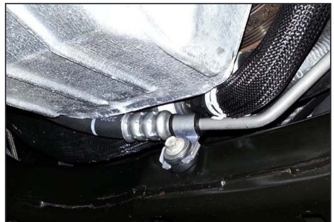
Power Steering Line Bracket's New Location
