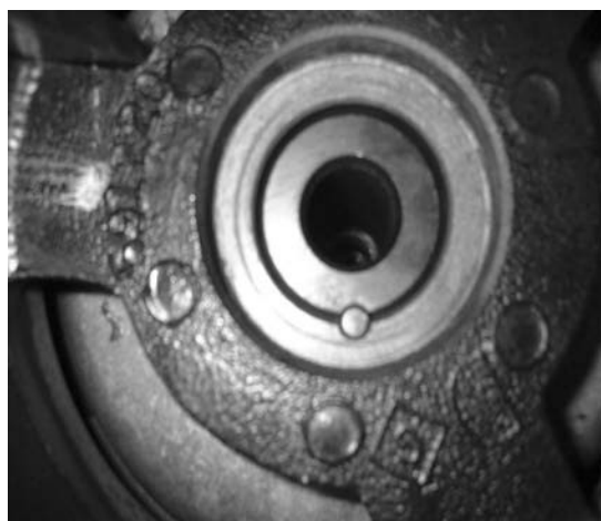
Crank Pulley Pinned to Crankshaft
