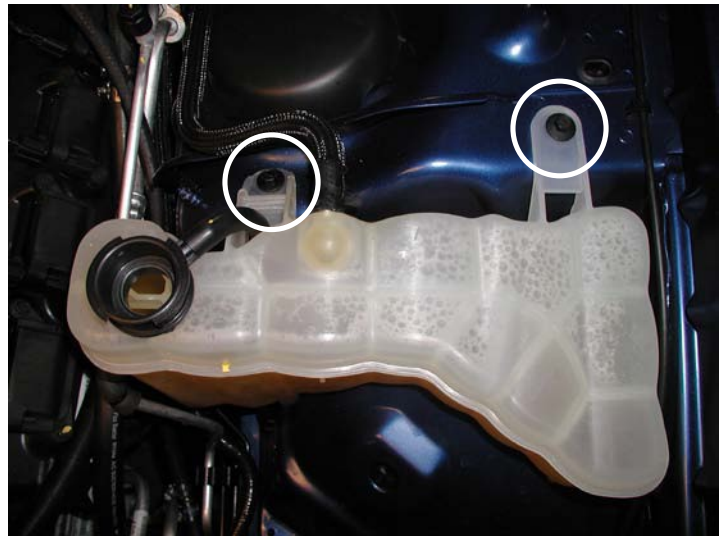
Remove Coolant Reservoir Bolts
