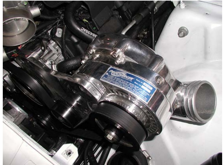
ProCharger Head Unit Installed
