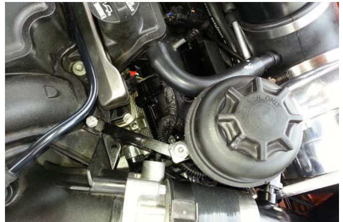
PCV Line Run To Air Inlet
