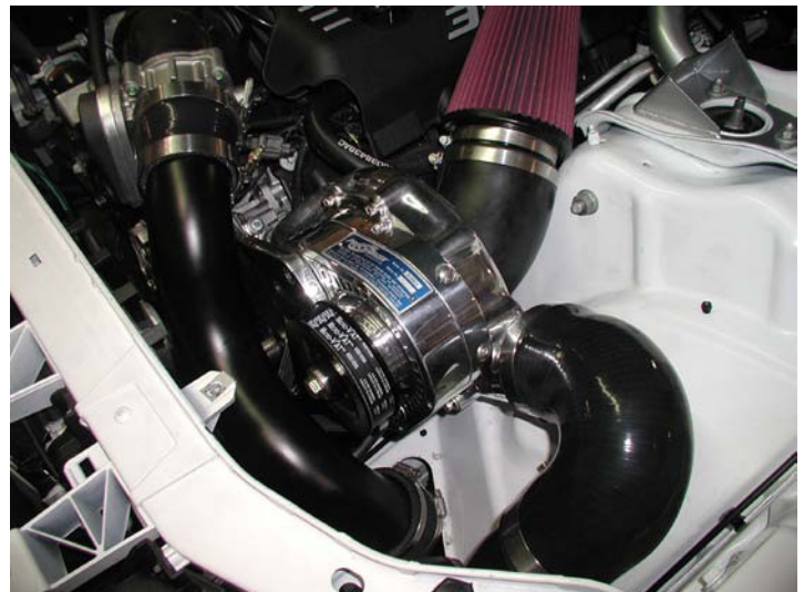
Throttle Body Tube (#315) Installed
