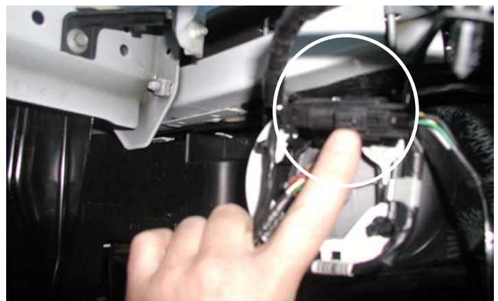
Disconnect Front Fascia Wiring Harness
