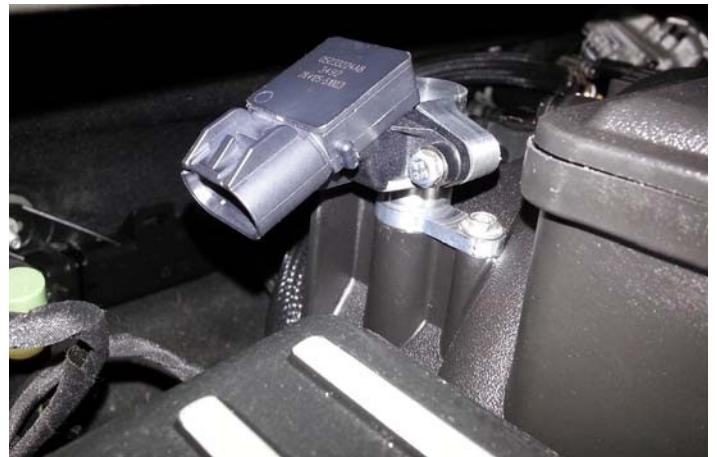
New MAP Sensor Installed
