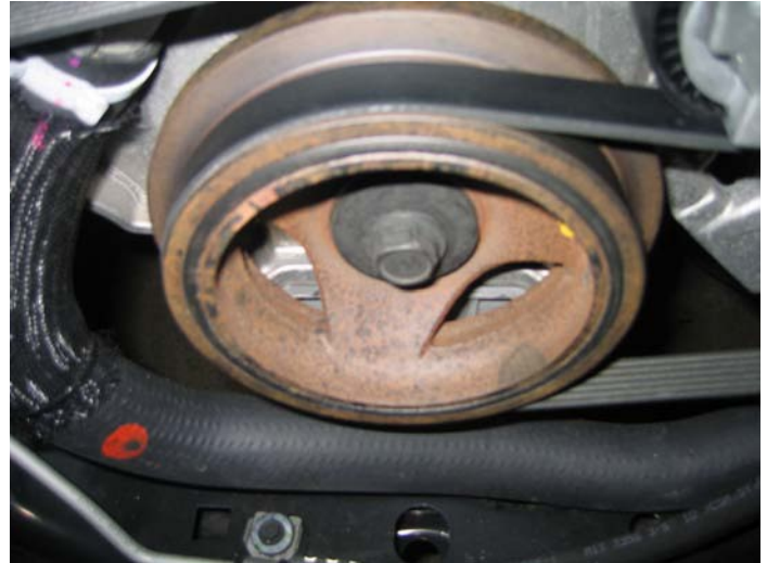
Factory Crank Pulley and Bolt
