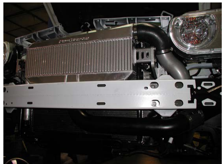
Stage 2 Intercooler and Tubing Installed
