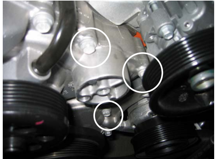
Remove 13mm Bolts For Sub-Bracket Install
