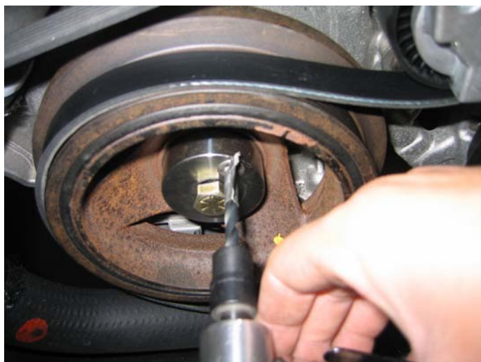
Drilling the Crank
