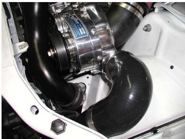
Blower Discharge Connection
