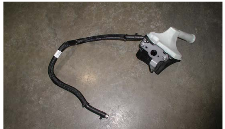
Power Steering Reservoir & Line Removed
