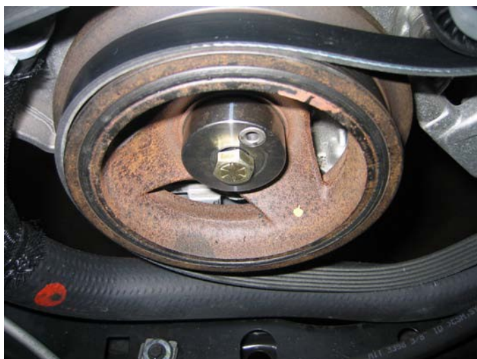
Drill Jig Installed
