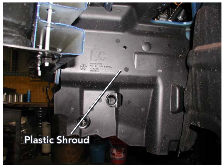
Driver's Side Plastic Shroud Removal
