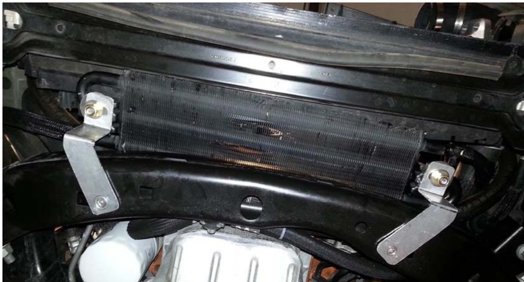
Relocated Power Steering Cooler
