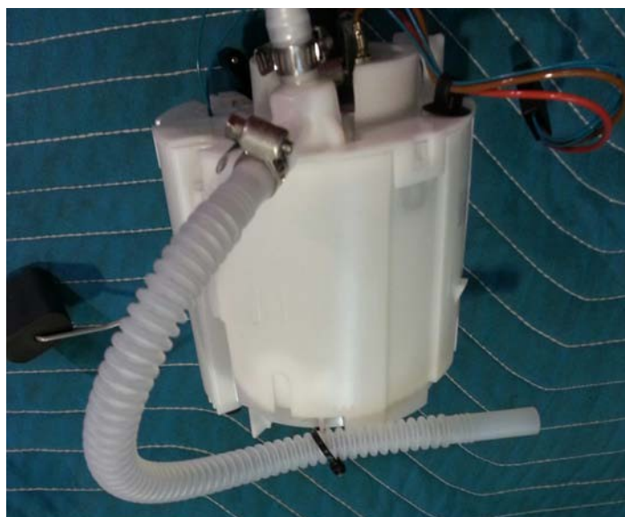
Suction Hose Attached to Basket
