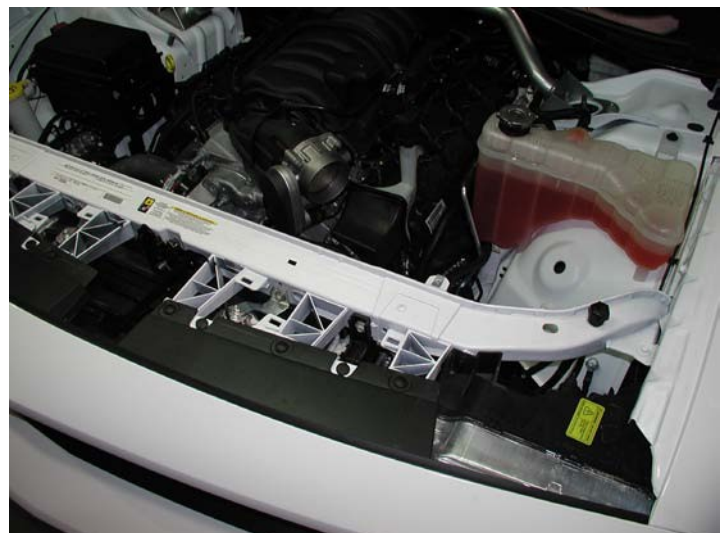
Air Filter Assembly/Cavity Covers Removed
