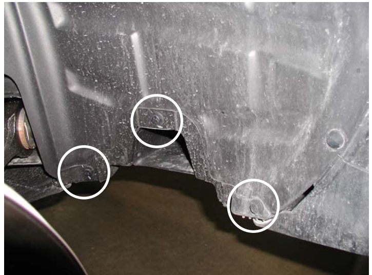
Front Fender Well Panel Fasteners
