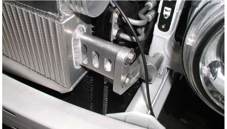
Driver's Side Intercooler Brackets
