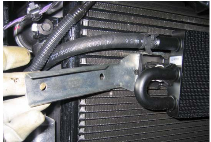
Power Steering Cooler Removal
