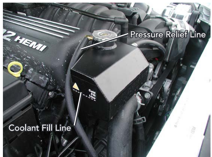
Pressure Relief Line Routing and Fill Line
