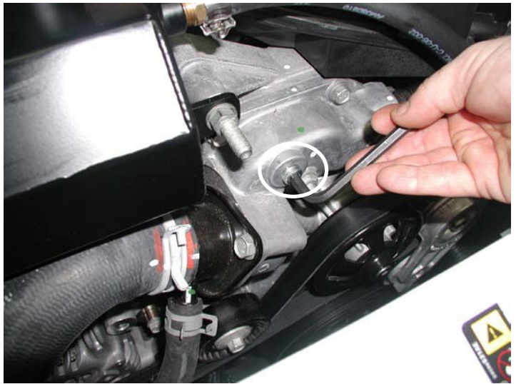
Cooling System Purge Screw
