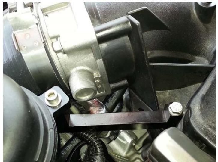
Lower Reservoir Bracket Mounting Location
