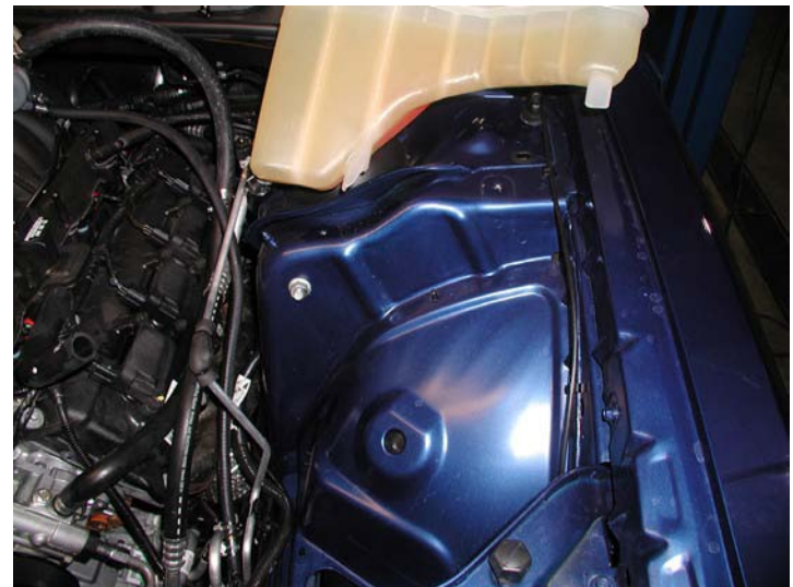
Lift Reservoir Out of Way
