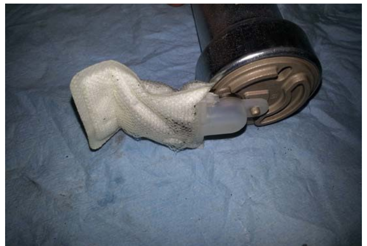
New Fuel Sock Installed
