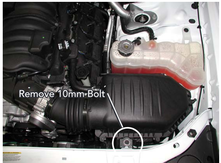
Remove Air Filter Assembly Bolt
