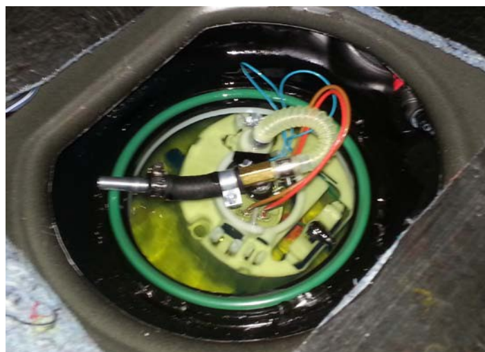
Pump Assembly Into Tank
