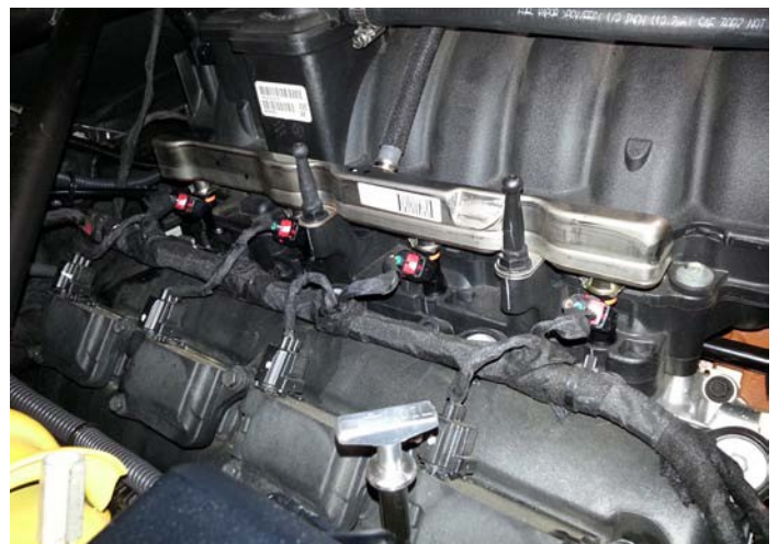
Fuel Rails Installed
