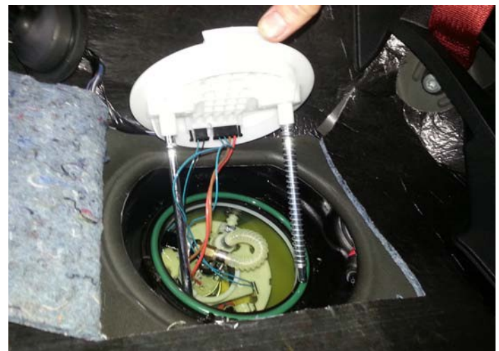
Electrical Connectors Under Pump Lid
