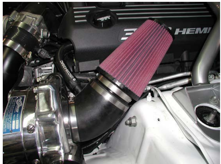
Air Inlet Assembly (With Upper Strut Brace)
