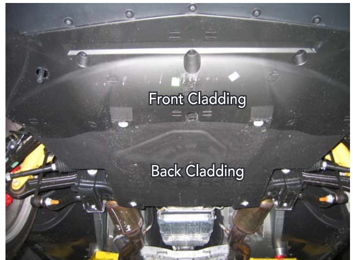
Underside Body Cladding
