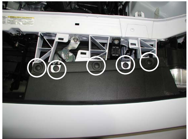
Top Fascia Connections (Driver's Side)
