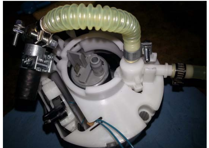
Jet Siphon Installed in Basket
