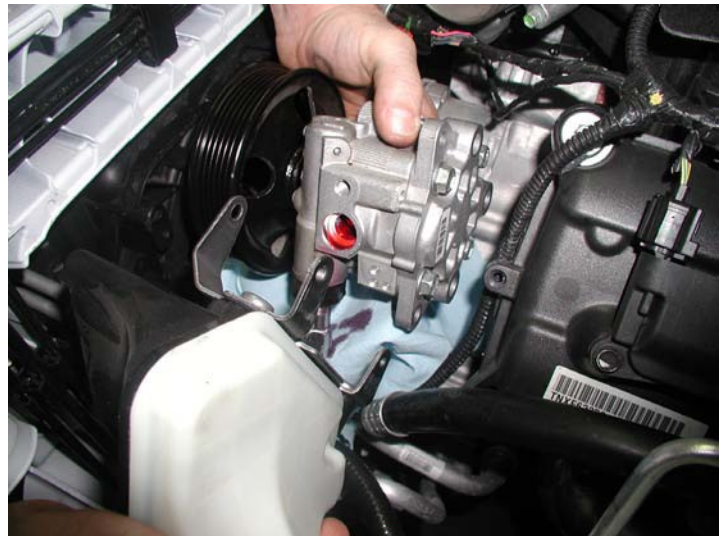
Power Steering Pump & Reservoir Separated
