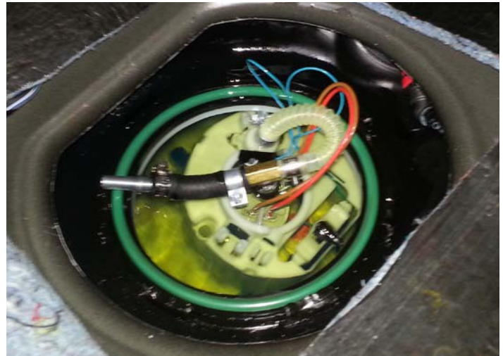
Pump Assembly Into Tank
