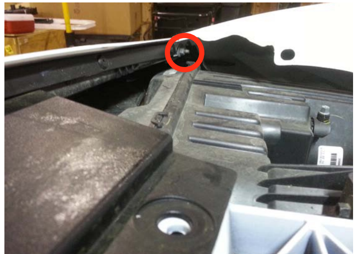
Upper Fascia Nut (Passenger's Side)
