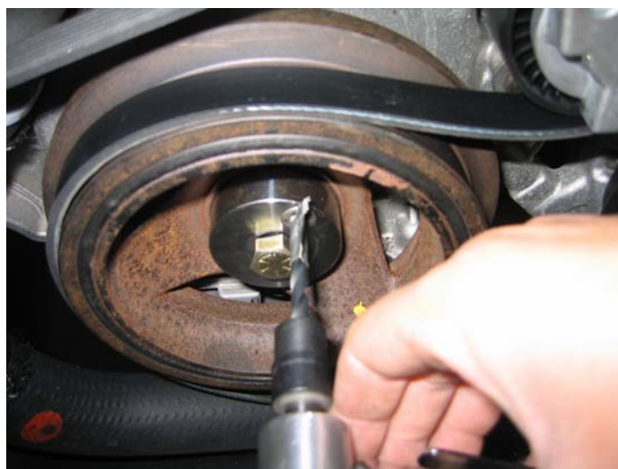
Drilling the Crank
