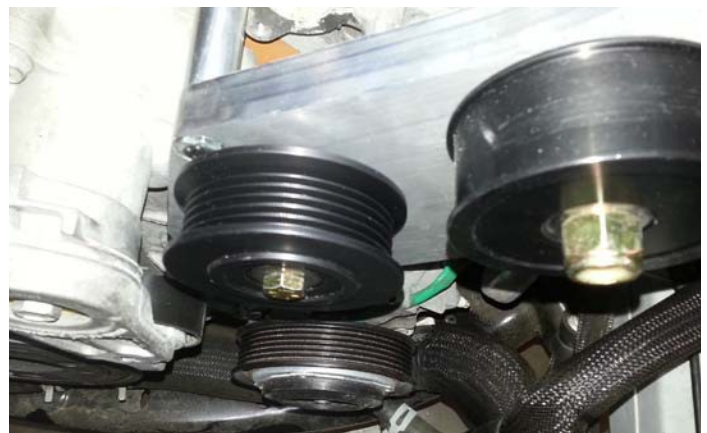
Ribbed Idler Installed
