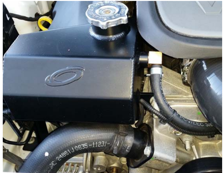
Coolant Hoses Connected
