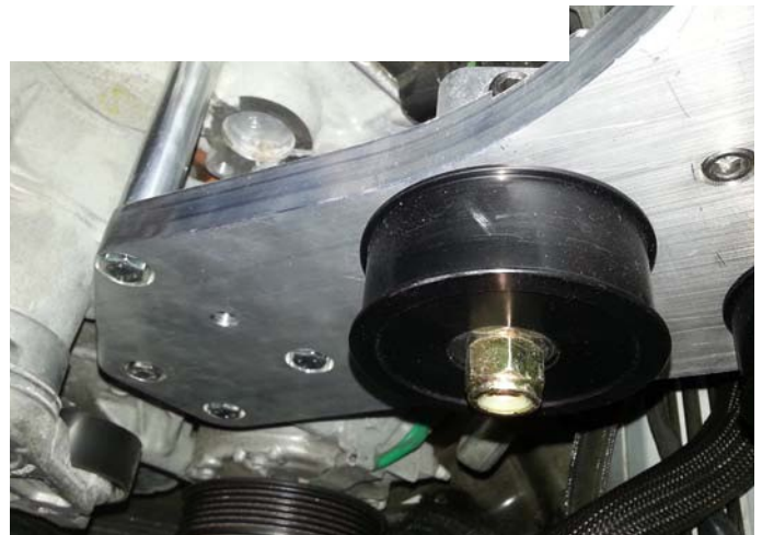
Main Bracket Installed
