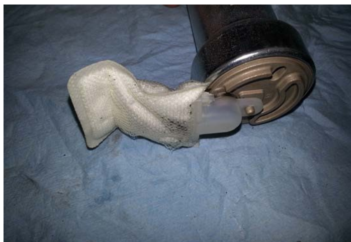
New Fuel Sock Installed
