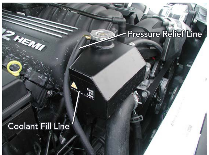
Pressure Relief Line Routing and Fill Line
