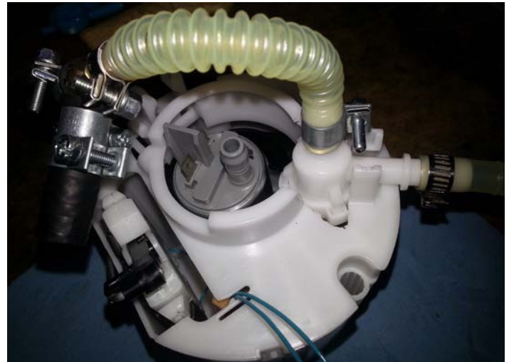
Jet Siphon Installed in Basket
