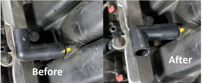
Locate mounting location for bracket. Depending on year of your vehicle, this hole maybe empty or have a plastic pin in it. If there is a pin in it, remove pin by wiggling it outward. Mount bracket with mounting bolt here.
